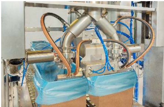
CIP cleanable, high accuracy weigh filling station
