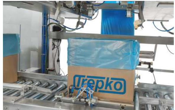
Cross sealed bag bottom and seal check for maximum bag integrity
