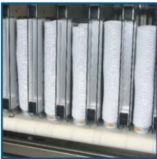
ergonomic cup stack feeding magazine
